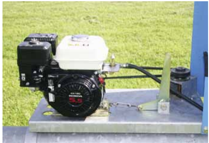
The 5.5 HP Honda® engine drive provides a cost effective mechanized irrigation option.
